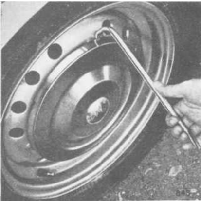
Fig. 17. Removing nave plate.
