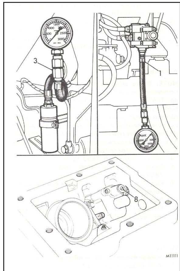
Start the engine and, using the Auxiliary lever, adjust the pressure valve screw until the desired pressure is obtained. Stop the engine and re-stake the screw. Remove the wire retaining the spool valve. (If the desired pressure can't be achieved there may be an internal leakage fault)
