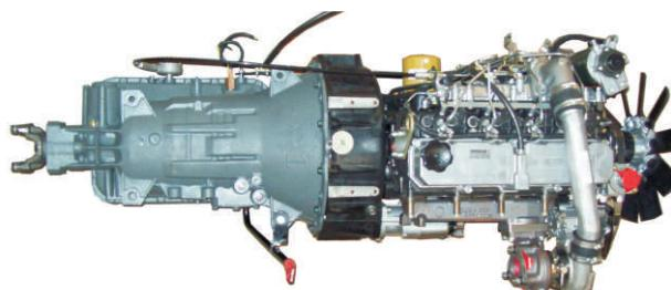
Transmission shown mounted on a Mitsubishi S4S-DT engine.
