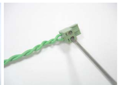
Figure 1.18 - Tighten the screw to secure the perimeter wire into the connector
